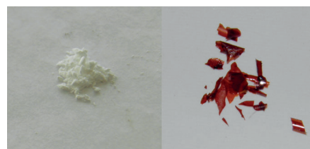
Figure 5. Visual appearance of polymer 10 (left) and its film composite with C_{60} (right).
